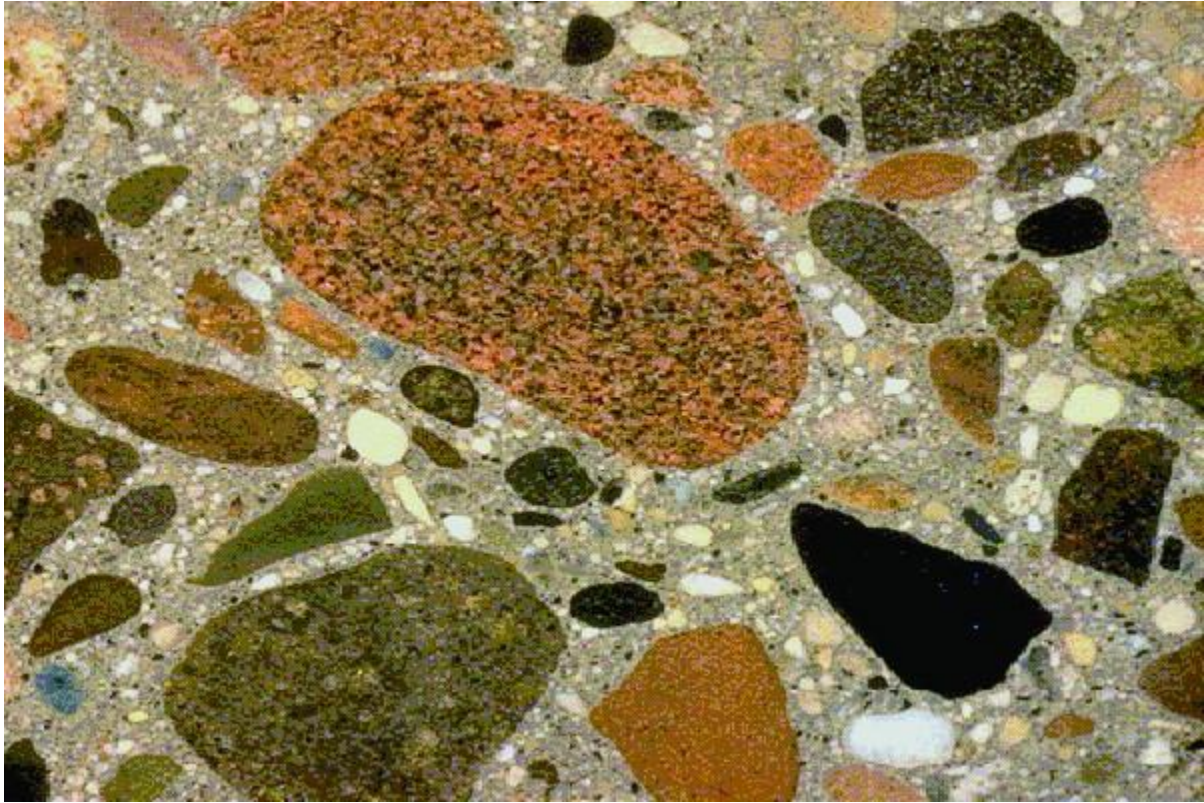
Figure 1 - Aggregate (75%) + Cement (25%) + Water
